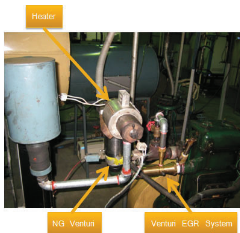
Fig. 15. Venturi EGR system on the in the intake manifold
